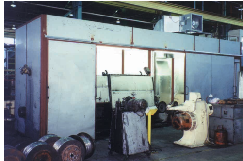
Large localised enclosure constructed in-situ in cable making factory
